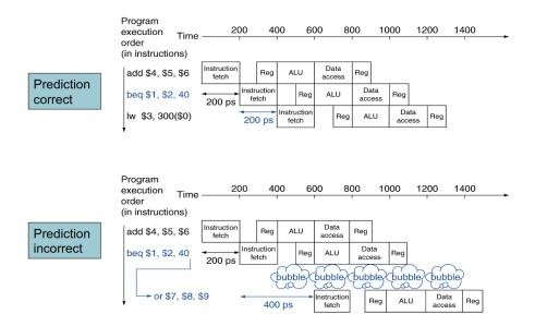
Thus when the pipeline makes the wrong choice for its branch prediction we stall for one cycle (if we don't make a prediction we would always need to stall for one cycle)
